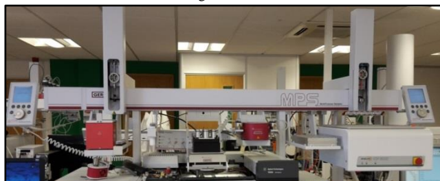
Figure 1: GERSTEL Dual Head MPS for fully automated Folch extraction and direct derivatisation
