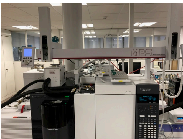
Figure 1 – GERSTEL Dual Head with Agilent GC/Q-TOF with large volume injection on CIS.
