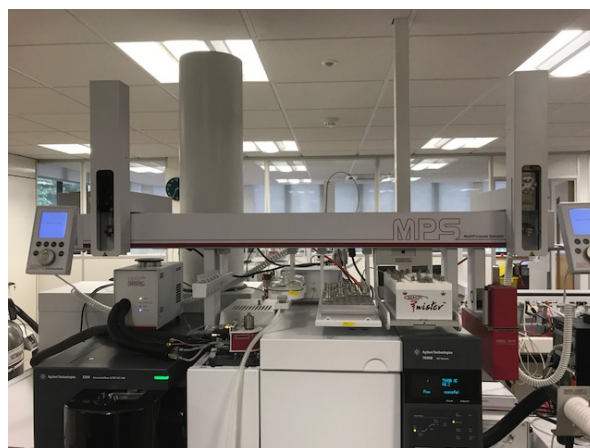
Figure 2 shows the GERSTEL Dual Head with Thermal Desorption on Agilent GC/QTOF at Anatune
