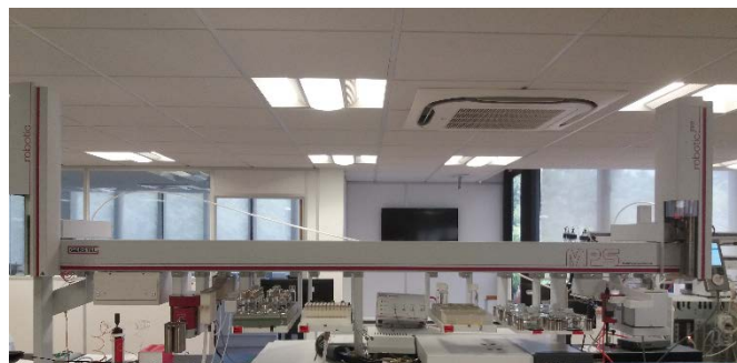
Figure 1. GERSTEL Dual Head Robotic MultiPurpose Sampler, mounted to an Agilent GC-MS
