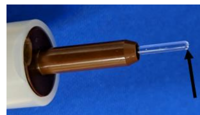
Figure 5. Round tip probe with a very small amount of tablet scrapings on the tip, which is enough for sampling with direct insertion GC/MS.
