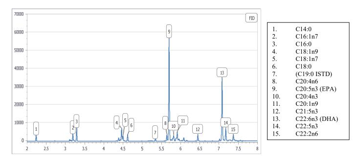
The MIDI Sherlock enhanced analysis software can automatically categorize compounds by type. Based on the label of the two fish oils analyzed, the samples passed the specification for EPA, DHA and total Omega-3 fatty acids, as shown in Table 2.
