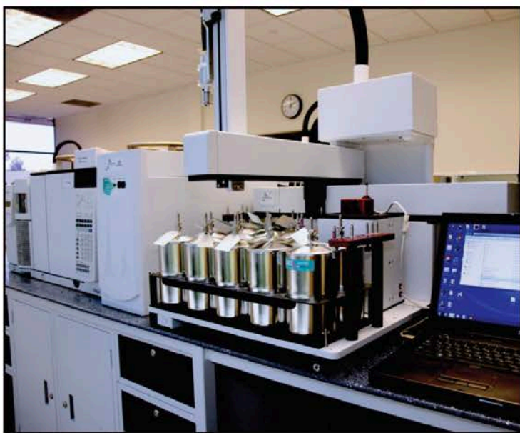
Figure 2 The 7650-M/7200 was used for this study on an Agilent 7890/5975. The 7650-M is the only multi-canister autosampler available that uses a single inlet to analyze all canisters, with only momentary contact being made in order to maximize recovery and minimize carryover.
