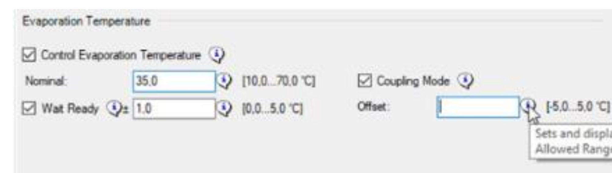
Figure 1. Screenshot of the part in the instrument method to activate the Temperature Coupling Mode and set the offset between EvapT and CDM temperature in a range of -5° C to +5° C
