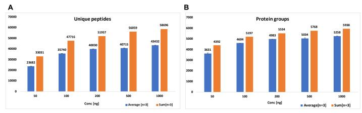
Furthermore, the performance of the Orbitrap Exploris was evaluated with variable gradients both in DDA and DIA experiments. For these experiments 200 ng HeLa digest was injected on column and separate with 5min (8min in total), 13 (15min in total), 20min (23min in total) and 44min (46min in total) gradients Figure 3 A and B shows consistence identification even at short gradients of 5min (>6000 peptides and 1000 protein aroups).
