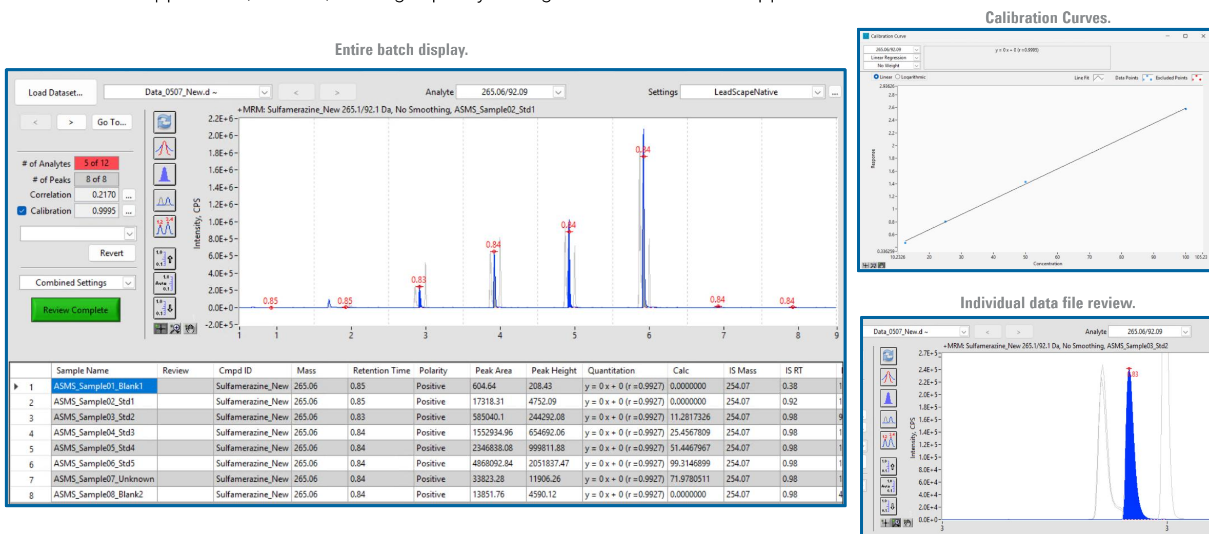
Figure 3. Easy to review individual chromatograms vs entire batch and calibration curves.
