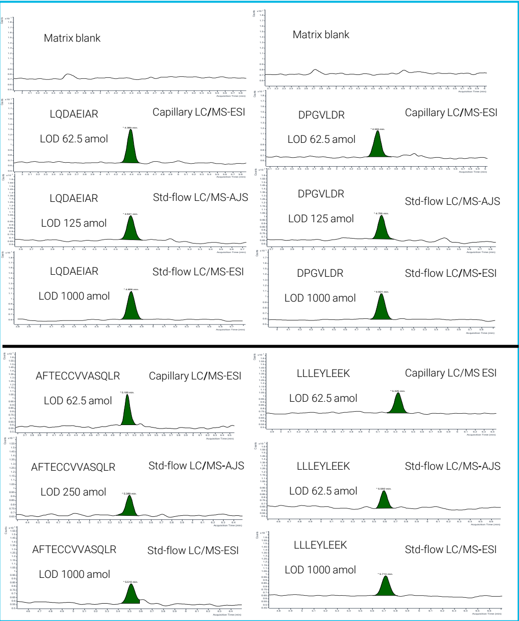
Figure 5 Stacked extracted ion chromatograms showing the LOD
