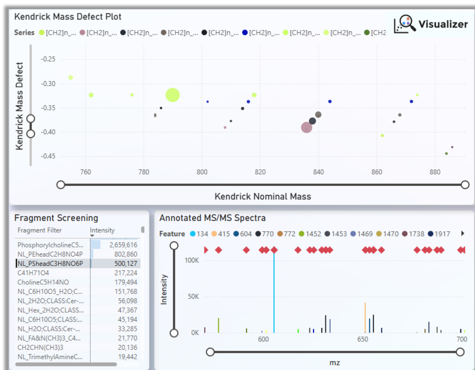
Figure 5. LipidMatch Visualizer zoomed view of the Kendrick Mass Defect Plot. The neutral loss (NL) corresponding to the PS headgroup was used to filter features indicating PS lipids.
