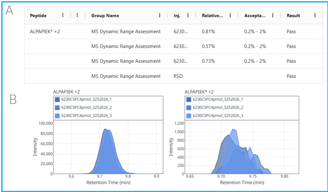
Figure 5. (A) Automated evaluation of the peak area ratio for ALPAPIEK and its isotopically labeled analog ALPAPIEK* (Lys- 13 C 6 , 15 N 2 ) measured at 4 pmol on column and compared against predefined acceptance criteria to confirm adequate MS dynamic range. (B) EICs of the ALPAPIEK and ALPAPIEK* peptides demonstrate consistent signal response and robust feature extraction.
