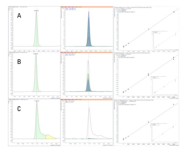
Figure 3: MassHunter Quant 12 images of the quantifier (left), qualifier(s) (center) and calibration curve (right) with the low end featured in the inset. (A) *N*-acetyl-L-glutamic acid, (B) Glycerphosphocholine, (C) ATP all show good linearity across an extended dynamic range.
