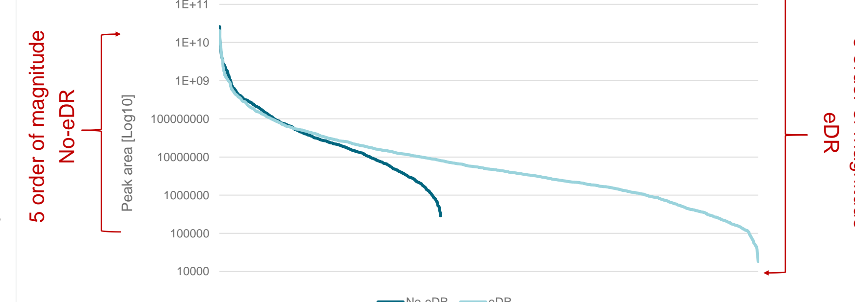
Figure 11. A regression of all compounds found in the above graph via MS1 are plotted with m/z on the X-axis and peak area on the Y-axis. This shows how eDR expands the compound dynamic range to 6 orders of magnitude.
