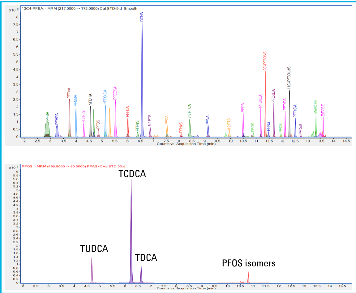
Figure 2. MRM chromatograms for all PFAS targets, EIS, and NIS compounds (top), and PFOS isomers and cholic acids interferences. (B)
