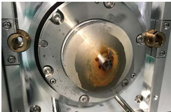
Sweep cone after 4000 injections
