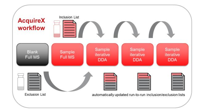
Compared with Traditional DDA, AcquireX Deep Scan Workflow Significantly Increases ID by Triggering More MS/MS and MS<sup>n</sup>
