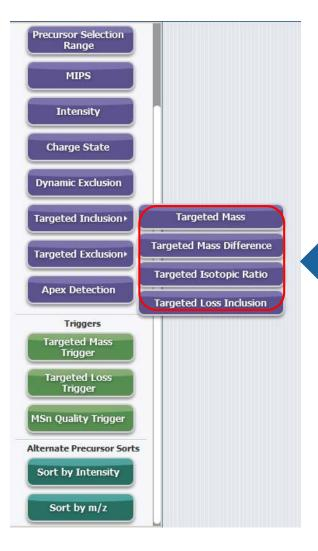
The feature-specific filters in ID-X method editor allow user to build sophisticated instrument method to capture trace level metabolites present in complex matrices, triggering MS<sup>n</sup> for confident identification and structure elucidation.
