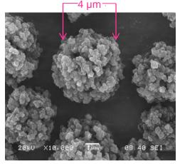
SEM Image of 4 µm Supermacroporous Bead
