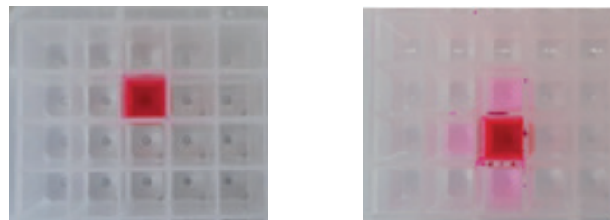
Figure 5a. 0.5 and 0.75 mL volumes mixed in a 1 mL/well nominal volume square collection plate (Vortex Genie, setting 3) showing potential cross contamination when max fill volume is exceeded.
