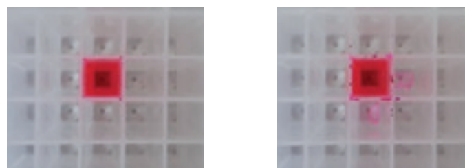
Figure 5b. 1.5 and 1.75 mL volumes mixed in a 2 mL/well nominal volume square collection plate (Vortex Genie, setting 3) showing potential cross contamination when max fill volume is exceeded.
