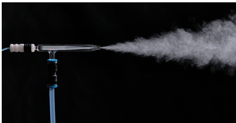
A nebulizer turns the liquid sample into an aerosol.
