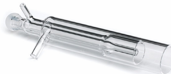
The plasma is formed from argon gas flowing in a quartz tube.
