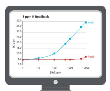
As the concentration of Na increases in a sample, the recovery of K can get worse. The impact is pronounced when viewing the plasma in axial viewing mode.
