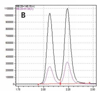
Fig. 2 Chromatograms obtained after an injection of a 5  $\mu$ L whole blood extract spiked at 200  $\mu$ g/L. Order of retention - A: norephedrine and norpseudoephedrine /B: ephedrine and pseudoephedrine
