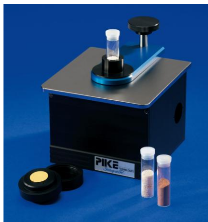
Figure 4. IntegratIR NIR sampling accessory. Samples or sample containers are placed on the integrating sphere for analysis. There is no sample preparation required or cleaning of accessories surface between analyses.
