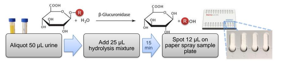
IMCSzyme®RT recombinant β-glucuronidase, buffer, and internal standard solution were combined in one spiking solution to minimize sample handling. The automated paper-spray sample cassette holds 24 samples. 240 samples could be processed automatically per run at 2 min/sample. Analysis was carried out using the VeriSpray™ paper spray system coupled to a TSQ Altis™ triple quadrupole mass spectrometer.
