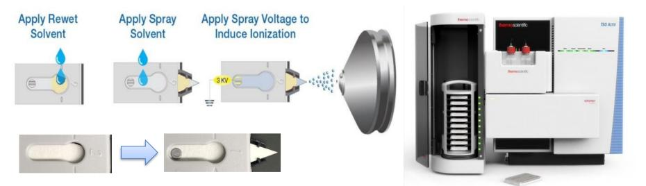
Figure 1 and 2. (Left) Paper substrate extending towards MS inlet prior to voltage onset. (Right) Thermo Scientific<sup>™</sup> VeriSpray<sup>™</sup> PaperSpray ion source. Thermo Scientific<sup>™</sup> TSQ Altis triple quadrupole mass analyzer
