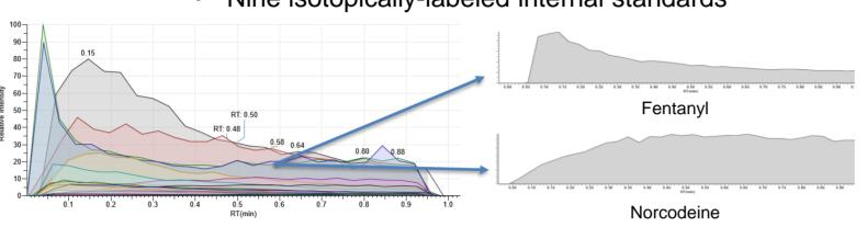
Figure 3. Paper spray chronograms depict elution profiles of target compounds Data was analyzed using TraceFinder 3.3 (Thermo Fisher Scientific). Positive results were considered valid if primary and secondary transitions were present in a pre-established ratio. Isobaric interference yielded failed ion ratios and an inconclusive result
