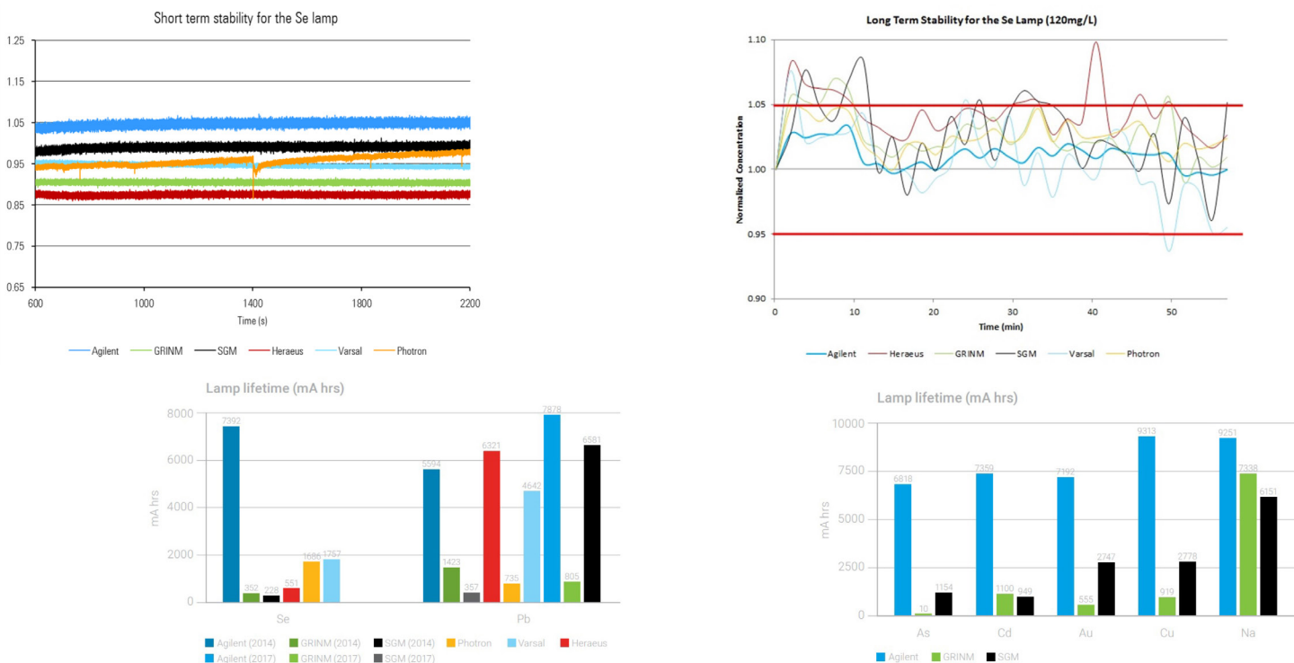
Figure 3. Performance of Agilent HC lamps. Short term stability measured after a 10 minute warm-up, and long term stability determined by reading a standard that gave good S/N repeatedly over an hour. Lamp lifetime was determined by operating the lamp continuously until failure.
