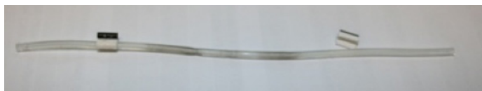
Figure 6. Change peri-pump tubing that looks or feels worn or has a strange colour. Ensure tabs are secure.
