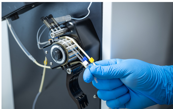
Figure 5. Easy-fit ICP-MS peristaltic pump tubing is optimized for the Agilent ICP-MS.
