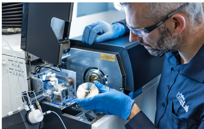
Figure 7. Visually inspect the cones.
