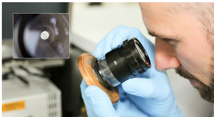
Figure 8. Agilent's LED measuring magnifier (5190-9614) is a tool to help users achieve optimum ICP-MS instrument performance and maximum cone life.
