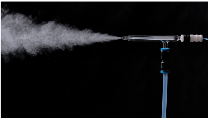
Figure 3. Micro-flow nebulizer aerosol.
