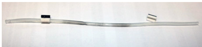
Figure 3. Extreme example of worn, discolored peristaltic pump tubing.
