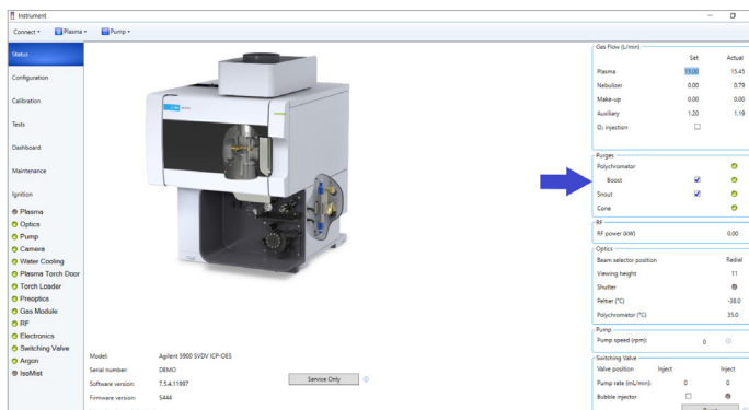
Figure 2. Simply click on the check box next to "Boost" and wait for the green light to indicate the polychromator boost is enabled and stable.
