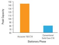
Sharper peaks result in a significantly higher peak capacity for 150-C18 compared to the conventional solid core C18 column.
