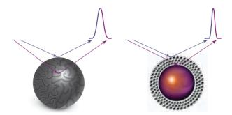
Resistance to mass transfer is minimized by the solid core design of Accucore particles as the diffusional path of analytes is limited by the depth of the
