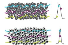
The tight control of particle diameter and automated packing process used for Accucore columns result in a tight, highly uniform packed bed that minimizes eddy diffusion.
