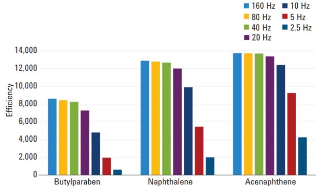
Fast data collection rates must be used with Agilent InfinityLab Poroshell 1.9  $\mu$ m columns to accurately measure the efficiency of the column, especially for early eluting compounds such as butylparaben (k' = 1.3).
