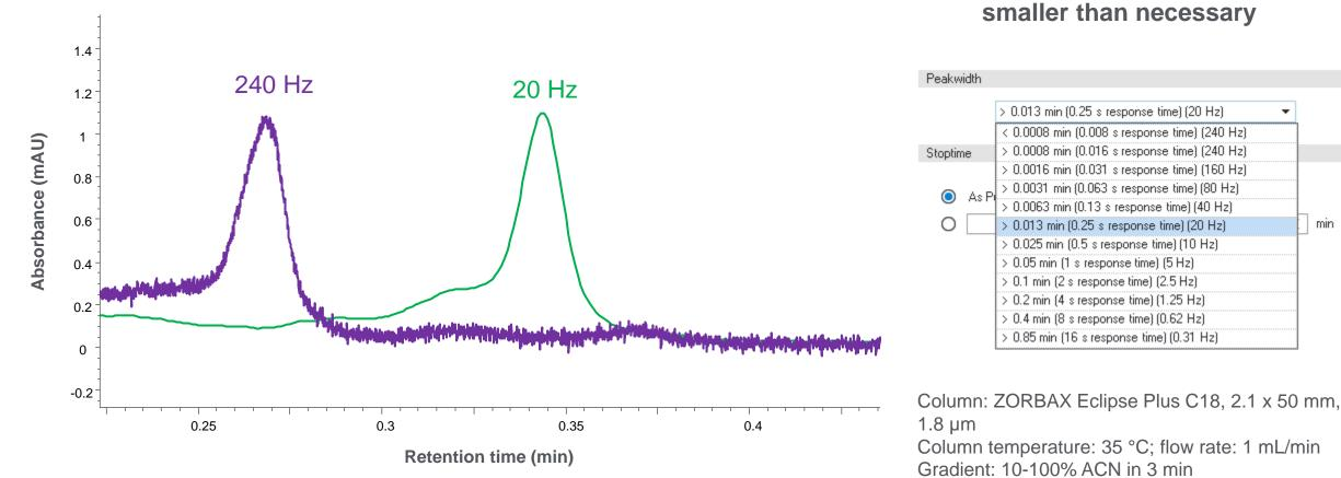
Signal: 254 nm, bandwidth: 4 nm Reference: 360 nm, bandwidth: 100 nm
