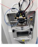
A 75 μm x 650 mm (P/N 6041.5775) "resistor" tubing is fitted between the ESI probe and ground to reduce the spray current and make it possible to utilize mobile phases with high ionic strength
