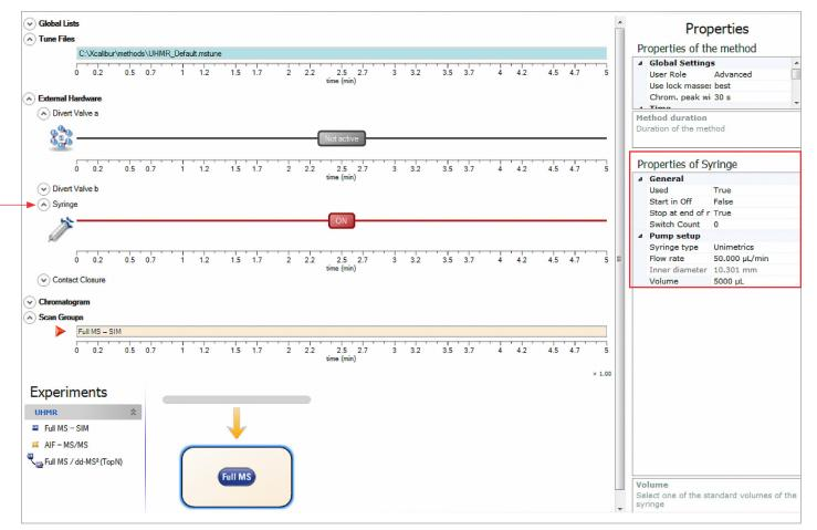
Figure 7. Q Exactive UHMR method with syringe drive control turned on
