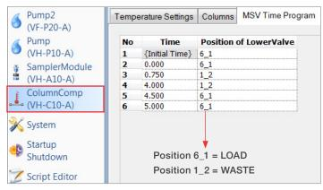
Figure 3. Time scheduling of the 2p6p valve switching from the instrument method editor
