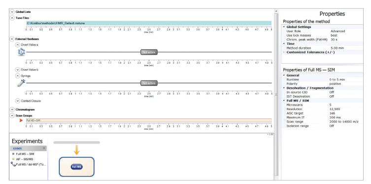
Figure 4. Q Exactive UHMR mass spectrometer standard method example for OBE Native MS
