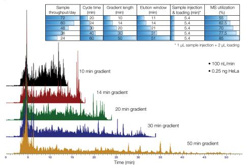
Figure 2. Five optimized LC-MS methods balancing sensitivity and throughput for different proteome coverage needs
