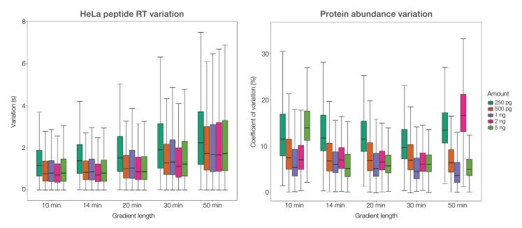
Figure 5. Low retention time variation and high quantitation accuracy of the LC-MS performance
