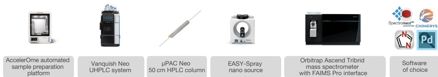
Figure 1. Graphical schematic of the Velocity LFQ DIA workflow for label-free quantitation on the Orbitrap Ascend Tribrid MS together with the optional AccelerOme automated sample preparation platform
