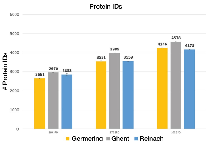
Figure 5. Inter-laboratory reproducibility of high-throughput LC-MS analysis. Proteome coverage obtained for 200 ng human protein digest standard across three sites and with three high-throughput methods, data processed with Spectronaut 18 software.
