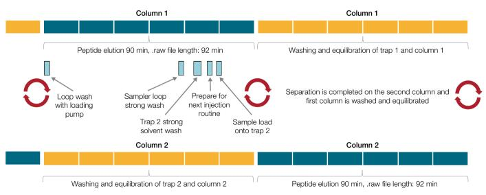
Figure 5. Schematic of the pre-concentration tandem high-throughput low-flow LC method
