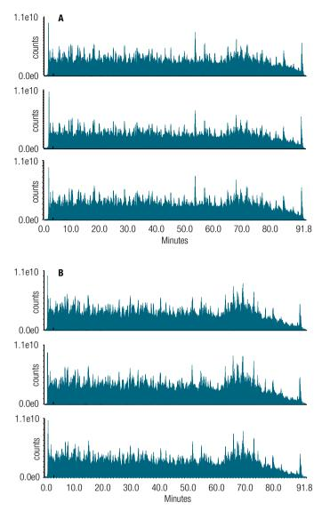
Figure 7. Typical TIC profile of HeLa protein digests for repeat 1  $\mu g$  injections on (A) trap 1 column 1 and (B) trap column 2, analytical column 2
