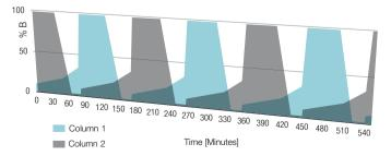
Figure 1. Flow-gradient schematic depicting the concept of tandem nanoLC operation. Note that the column wash phase, represented by an organic hold here for simplicity, is replaced by multiple "saw-tooth" wash cycles in the method described below.
