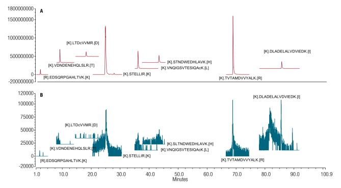
Figure 8. EICs for seven selected HeLa peptides from across the entire chromatographic range for both a 1 µg HeLa injection (A) followed by a blank injection (B)
