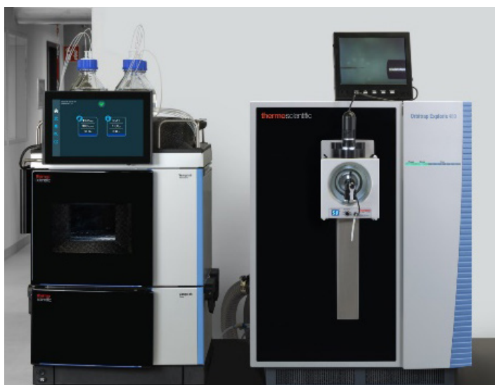
Figure 1. Vanquish Neo system coupled with the Orbitrap Exploris 480 mass spectrometer and scheme of direct injection workflow
