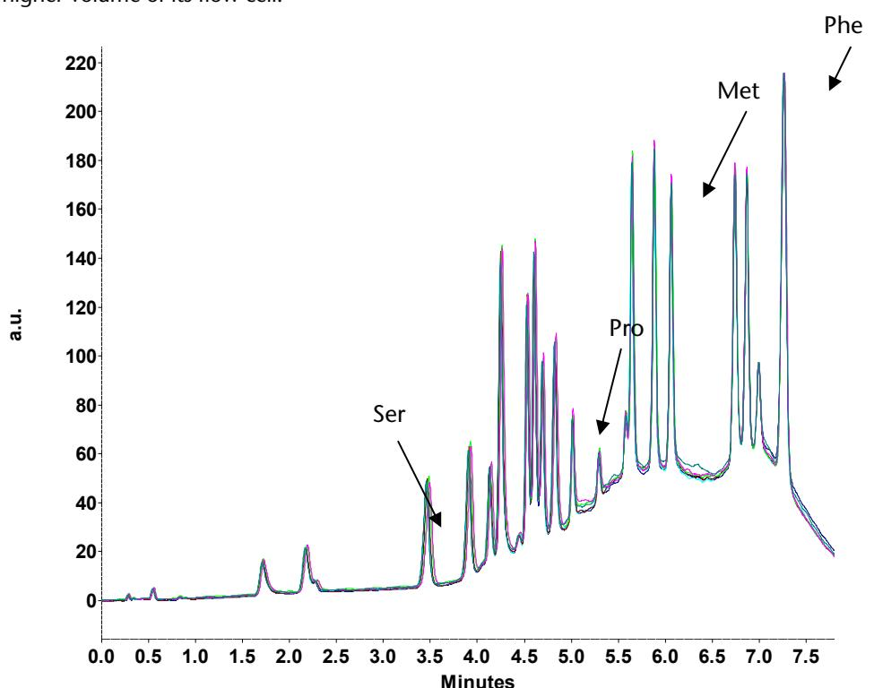
The overlay of five chromatograms in figure 5 shows the excellent reproducibility and robustness of the method. For a statistical evaluation, four peaks randomly distributed over the whole chromatogram were chosen as pointed out with arrows in figure 5. The statistical evaluation over the five replicate runs can be found in table 1.
