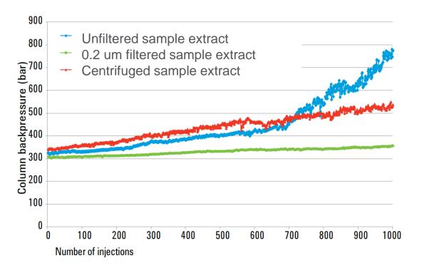
Unfiltered, centrifuged, and filtered sample extracts ZORBAX RRHD Eclipse Plus C18, 2.1 x 50 mm, 1.8 µm column, p/n 959757-902
