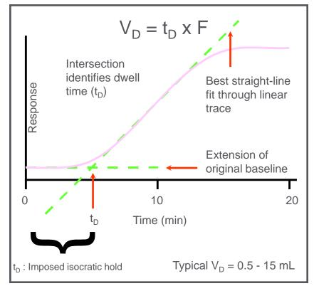
High pressure mixing:  $V_D$  = mixing chamber + connecting tubing + injector Low pressure mixing:  $V_D$  = the above + pump heads + associated plumbing
