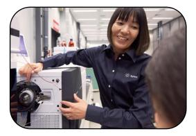
Check nebulizer spray, needle position, and clean the source
