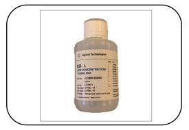
Run Checktune or calibration with fresh tuning mix
